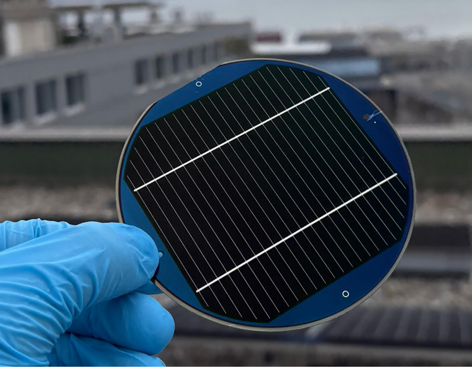
The triple-junction solar cell (54 cm 2 ). © Kerem Artuk
